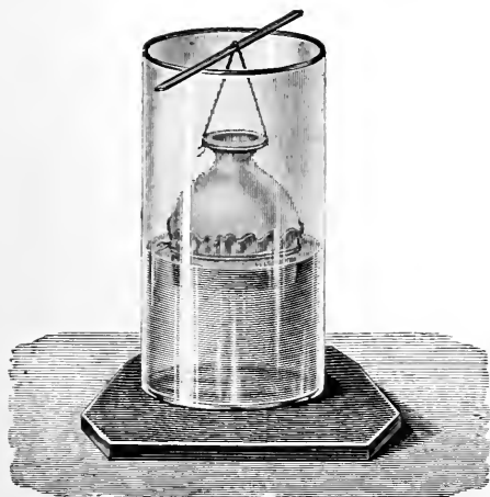
FIG. 6.—Dialyser. The lower opening of the bell jar suspended in water is tightly covered with parchment paper. The fluid to be dialysed is placed within this vessel, the crystalloids pass out into the distilled water outside, through the parchment paper.
